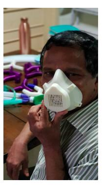
Picture 9: 3D printed N95 mask
